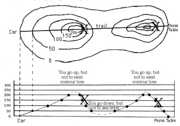
When the contour lines are close together, the slope is **steep.** when the contour lines are far apart, the slope is **flat.**
