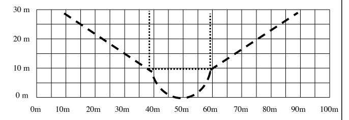
Cross Section Calculations: **Divide Plan B into 2 triangles and 1 half circle.**
