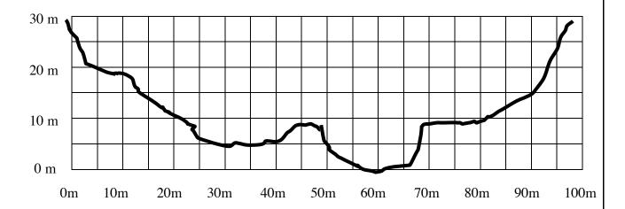
**Divide into Shapes.** Divide the cross-section into segments that are close to regular geometric shapes. In the diagram below; segments 1 and 3 approximate triangles, segment 2 is a rectangle, segments 4 and 5 approximate trapezoids, and segment 6 approximates a half circle.
